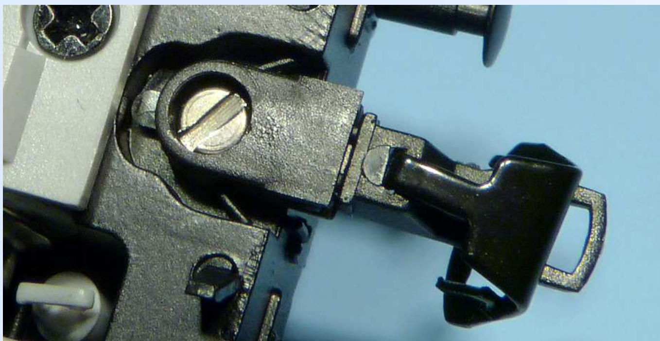
Obr. 23: Detail otočné šachty.
